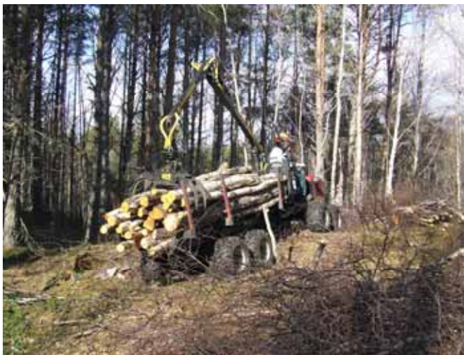
Extraction of the thinnings using a small forwarder helps gently scarify the ground and assists regeneration. Using a larger, less manoeuvrable machine would require the cutting of racks and would cause unacceptable ground damage on sensitive sites.
